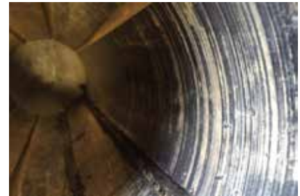
Abrasive wear on metal, select a grade with a higher hardness rating.
