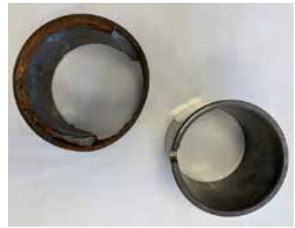
Cracking of carbon bearings
